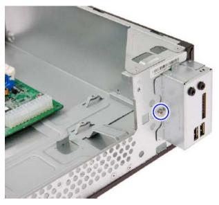
6. Pull the bracket out from the chassis.
